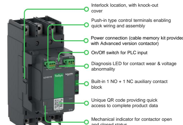
Contactors for TeSys Giga Motor Starter
